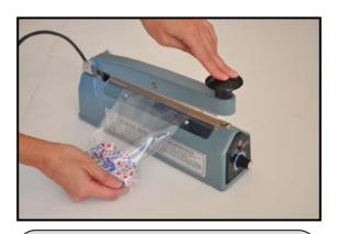
**Step 2.** Insert contents in bag. Place open end of the bag on the sealing pad.
