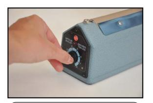
**Step I.** Plug in power cord and adjust timing dial to desired setting (a good starting point is  $2\frac{1}{2}$ ). For cut and seal (round element), adjust timer to the lowest setting that will still seal and cut.
