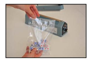
**Step 4.** Example of sealed bag. Cut and seal bags will not have bag material above the seal.
