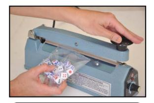
**Step 3a.** Cut and seal operations. While the sealing arm is depressed, tear the package away with your right hand.
