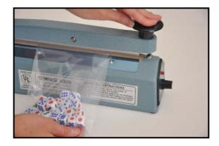
Step 3. To seal only, bring the sealing arm down (light pressure) on the bag and sealing pad. Keep sealing arm down until the red light turns off, plus an additional 2-4 seconds to set the seal.
