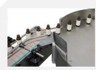
Level transition plate fits next to existing conveyor to facilitate easy transition from one conveyor to another
