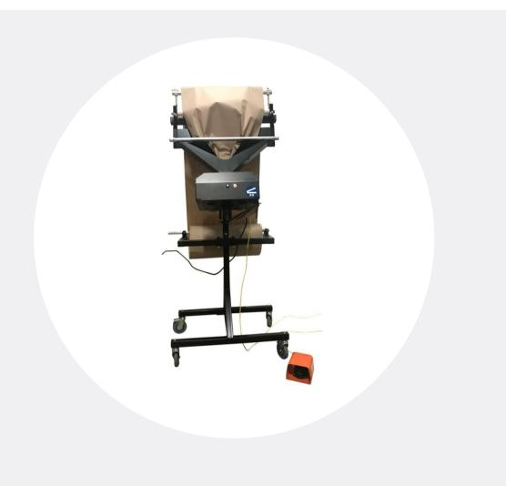
The SS-5980 Paper Dispenser with Crumple Device is simple and easy to use. Simply load the roll of Kraft paper onto the machine and feed the paper into the condenser where the paper is turned into usable void fill material used for packaging. The SS-5980 is designed for businesses who want to gain a big business advantage in protecting their products with limited space.
