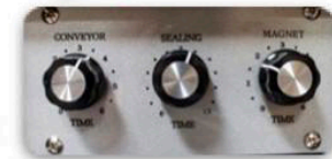
Sealer Control Panel
